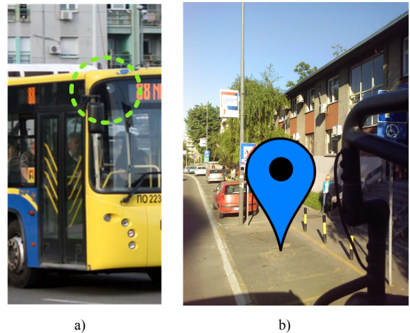
Fig. 9. Example 2 – a) Camera mounting position; b) one of the real camera snapshots taken from a mobile on-board-unit at 12m/s
