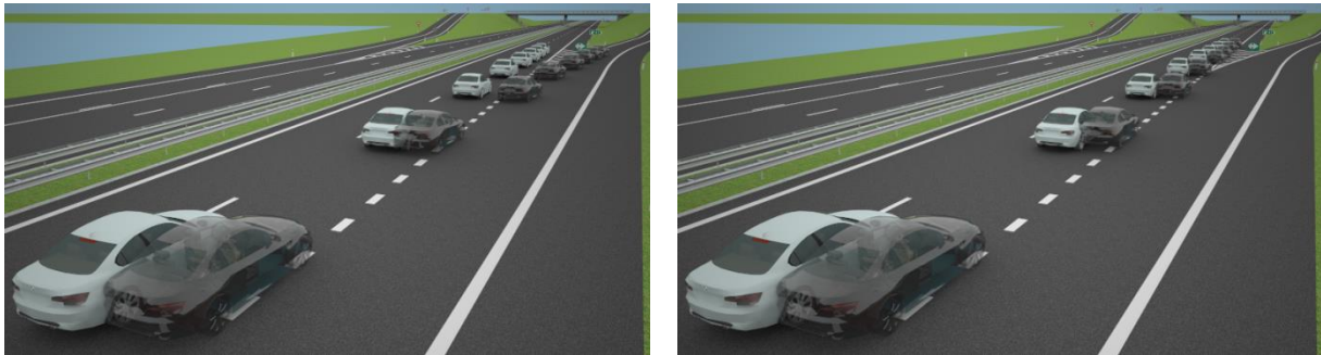
Figure 1: Left: Example of how current positioning systems may handle uncertain measurements. While the solid car is driving along a highway, the estimated vehicle position is mapped to the exit ramp where the AGD application would lower the velocity. Right: With the EAGD system the position of the vehicle is mapped to correct lane
