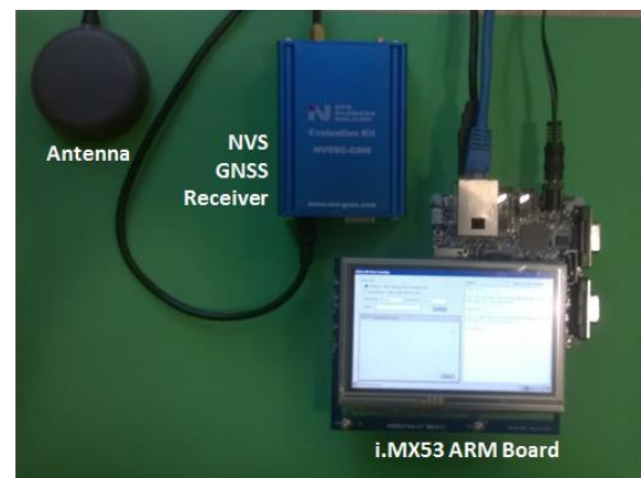
Figure 3. Embedded System Components
