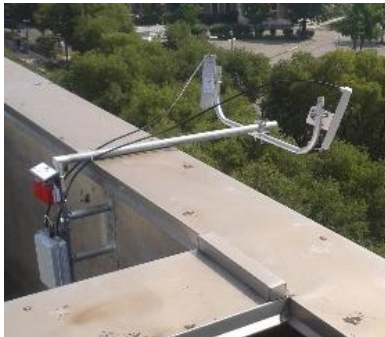
Figure 11 - Example of a real Road Side Unit equipped with two sectorised antennas
