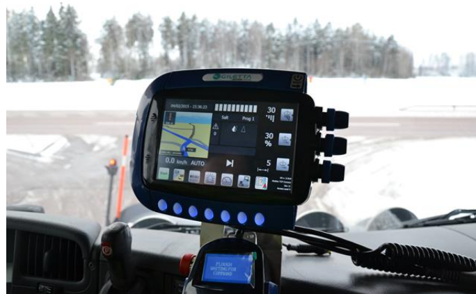
Figure 16: OBU shows pre-loaded geo localized information along the path according to the position (in this case, the road width and slope).
